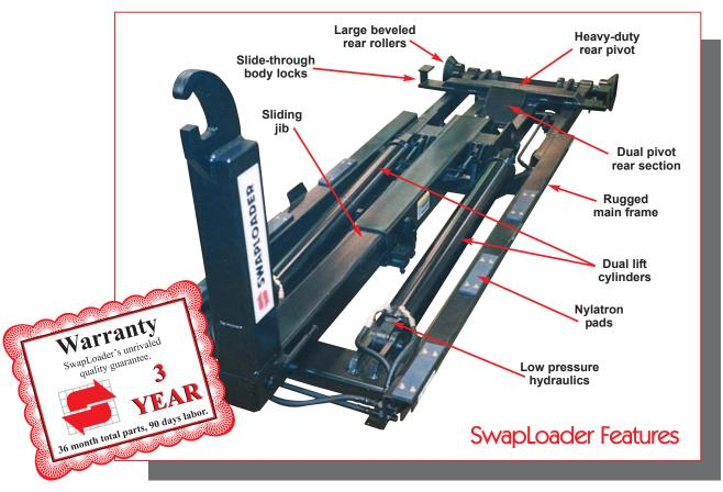
SwapLoader operates as a mount/dismount system and as a true dump truck. A high dumping angle assures the user of the ability to dump any and all loads quickly and efficiently. SwapLoader hoists include a safety valve to prevent jib operation in dump mode.
